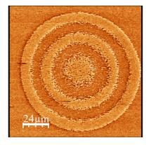
Figure: Domain structure stabilised after a single laser pulse of 5 ps. Image obtained by magnetic force microscopy. The orange (respectively brown) areas correspond to domains pointing upwards (respectively downwards) perpendicular to the plane of the sheet/screen. [1] E. Beaurepaire, J.-C. Merle, A. Daunois, J.-Y. Bigot, Ultrafast spin dynamics in ferromagnetic nickel. Phys. Rev. Lett. 76, 4250 (1996).
