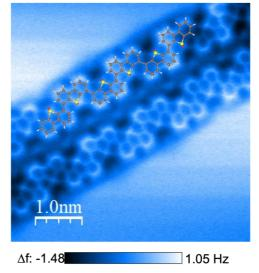
Atomic force microscopy image in non-contact mode with a CO functionnalized tip illustrating the on surface synthesis of dibromo-sulfoxide via Ulmann coupling obtained by annealing the molecular deposit on Au(111) surface at 200°C.(IM2NP,Marseille)
